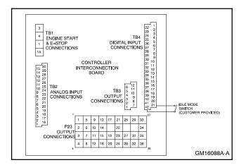
Figure 6-9 Idle (Speed) Mode Switch
